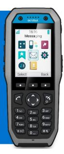
The Mitel 5617 IP-DECT handset is an enterprise-class handset that is designed for users who work in the toughest working environments. The Mitel 5617 is built to be comfortable to use throughout the longest shifts, featuring: a large color display, advanced messaging, wired or wireless headsets, multiple language and phonebook options, a carrying clip and a long-life, replaceable battery.
